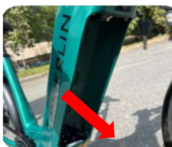
3. Hold battery carefully and lift out
