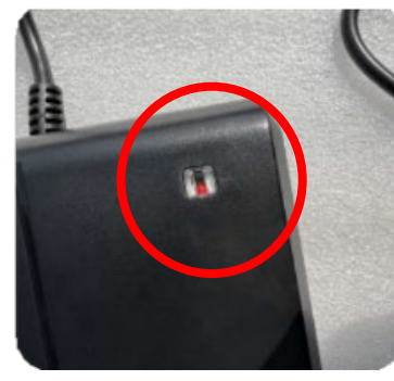
4. Red light shows the battery is charging, green light is full.
