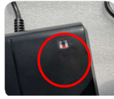
4. Red light shows the battery is charging, green light is full.
