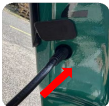
2. Charger hole in on the left side of the frame and near the folde.
