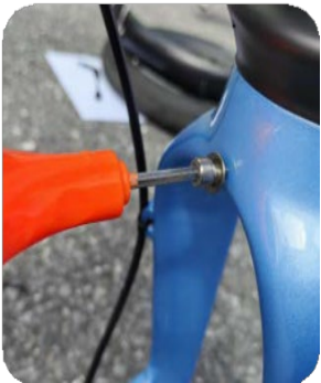
1. Fixing the front mudguard to the fork with screw
