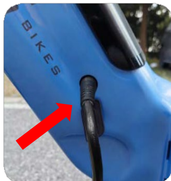
2. Charger hole in on the left side of the frame and near the handlebars.
