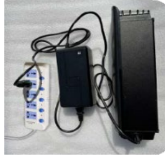
3. Plug one end of the charger into the battery & the other end into power supply.
