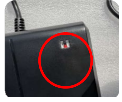
4. Red light shows the battery is charging, green light is full.
