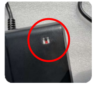
4. Red light shows the battery is charging, green light is full.
