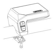
Then place the holding bracket on the underside of the display and tighten it into position with a M3.0\*8 screw. Torque requirement: 1.0 N.m.
