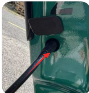
2. Charger hole in on the left side of the frame and near the fode.
