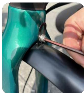
2. Fixing the front fender to the fork with screw. Fiber washer goes next to fork, metal washer next to screw head.
