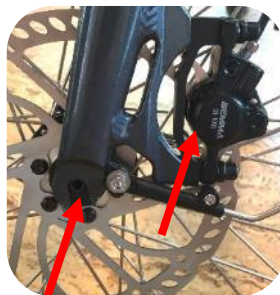
3. Insert the front wheel into the front fork ensuring the brake disc slides into the brake caliper opening.
