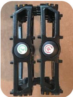
1. Pedals are marked for the Left and Right sides. The Left pedal is lefthand threaded, opposite the normal righthand screw and bolt threading
