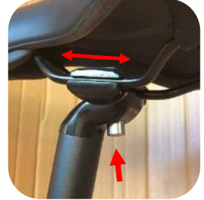
4. Further forward & back adjustments can be made by loosening the 6mm hex bolt under the saddle.
