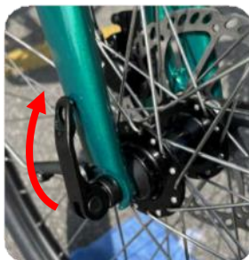
6. After tightening, push the quick release lever upward and check the operation of the wheel.
