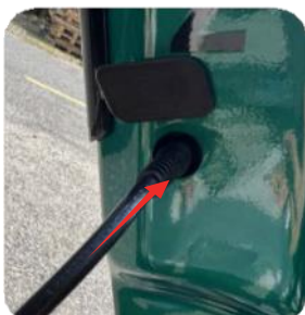
2. Charger hole in on the left side of the frame and near the folde.
