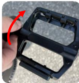
3. The right side pedal (R) is screwed in normally and tightened with the wrench in a clockwise direction.
