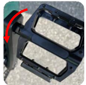
3. The left side pedal (L) is screwed in counter-clockwise and tightened with the wrench in a counter-clockwise direction.
