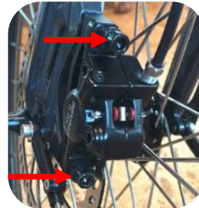
7. Off the ground, spin the front wheel and listen for any rubbing of the brake disc against the brake pads.
