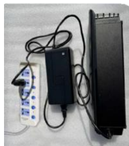
3. Plug one end of the charger into the battery and the other end into the power supply.
