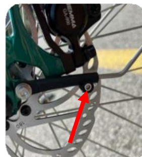
4. Slide stays out to provide room for wheel mounting.
