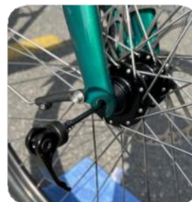
4. Insert the front wheel quick release clamp from the side opposite the brake caliper.
