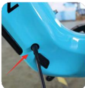
2. Charger hole is on the left side of the frame towards the bottom of the downtube
