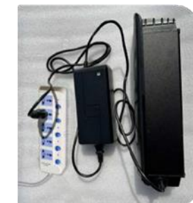
3. Plug one end of the charger into the battery and the other end into the AC power supply.
